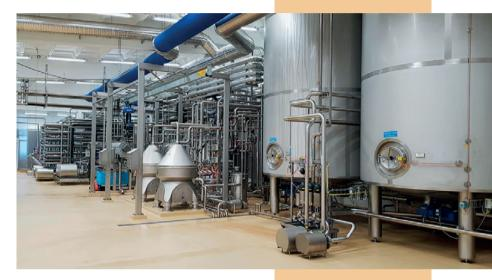
plier for automation and electrical installation for the wet mix plant as well as the existing CIP plant. The project is executed on Siemens S7 and Wonderware IAS, as HMI system. The delivery also contains MCC, remote I/O, frequency converters, and associated commissioning.
