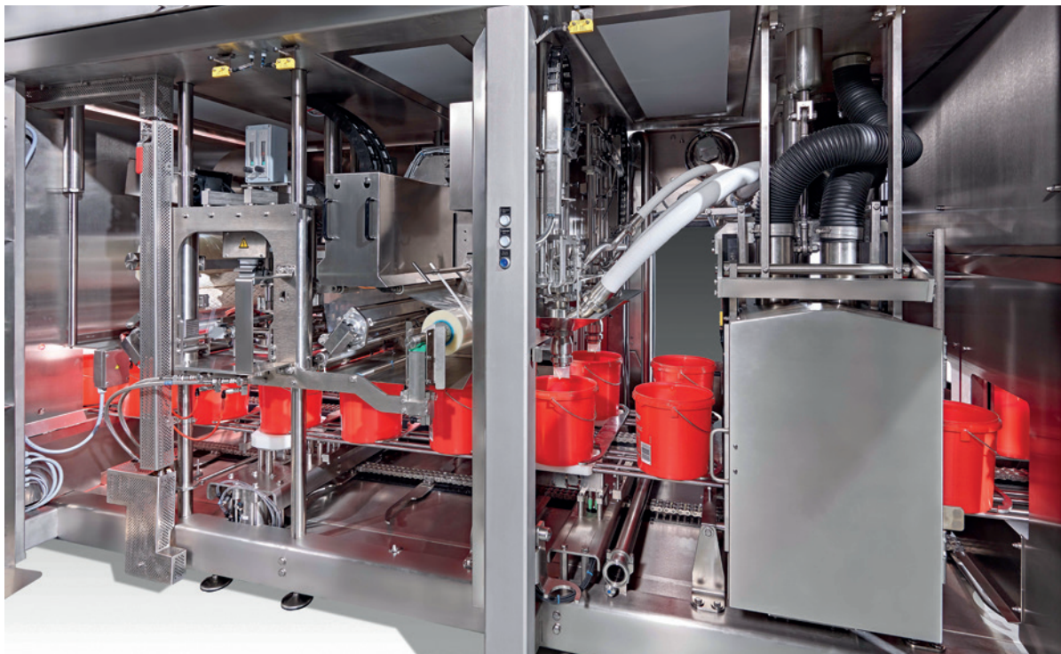
View into the inside of the inline bucket filler GRUNWALD-FLEXLINER XL UC: The ultra-modern UV(C) sterilisation area (on the right of the photo), filling station with weigh cell (middle) and cutting/sealing station with film sterilisation (on the left).
