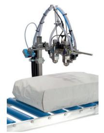
GRIP FIX anti-slip agents are watersoluble, solvent-free adhesives for securing pallet loads. The pallet loads may be PE bags, paper bags, cartons, cellophane-packed items, PP woven bags or small packages.
