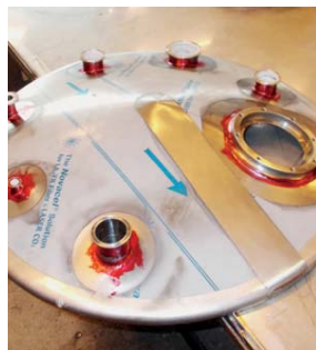
LP Kolding has recently delivered tanks to a Swedish customer in the Pharma industry, finalized with a test for Riboflavin and penetration. During the test the CIP nozzles in the tank are tested for critical areas for cleaning. The photo shows the penetration test.
