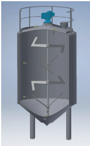
Skyr tank. The solid consistency of skyr imposes completely different requirements on the agitator than the skimmed milk. The agitator must touch the mass well so that it is completely uniform.
