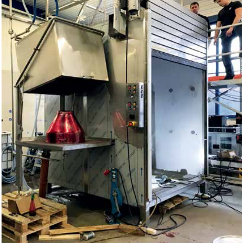
Cleaning cabin for transportable tanks.
