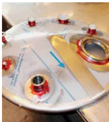
LP Kolding has recently delivered tanks to a Swedish costumer in the Pharma industry, finalized with a test for Riboflavin and penetration. During the test the CIP nozzles in the tank are tested for critical areas for cleaning. The photo shows the penetration test.
